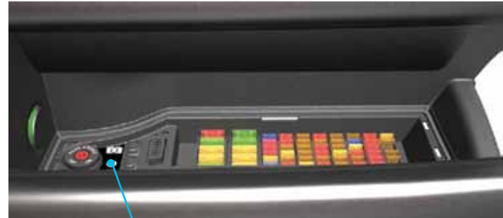
TPMS set (under the plastic panel)
