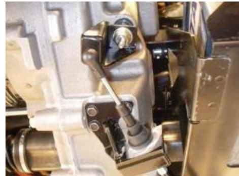
Disconnect Cable from Drive Unit
